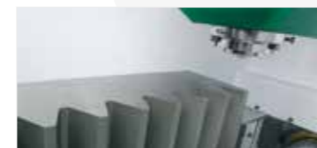
Collision protection system with the ability to detect impact forces of only 0.8 kg (8 N).
