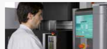
CNC-CAM capable of controlling up to 8 axes simultaneously, enabling CAD/CAM integration.
